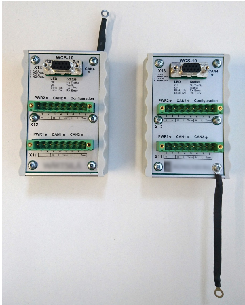
Figure 5: WCS-10 variants A (left) and B (right) with different ground strip attachment positions
