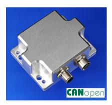
XY-CAN-EF is the 3-axis inclinometer sensor with CANopen protocol. The sensor can be used for measuring the lateral (X), longitudinal (Y) and vertical (Z) angle with respect to gravity. It can also simultaneously operate as a 360° (H) sensor in XY plane. Inclination measurings are based on the high accuracy accelerometer IC.
