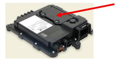
Depending of TGU-R ACCESS variant, a SIM card connector or an eSIM is available.
