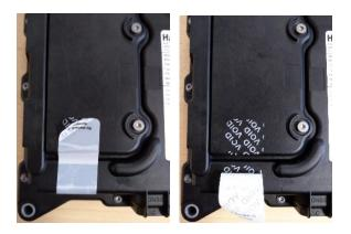
2- Once the inviolability label totally removed, put some isopropyl alcohol on a soft cloth, then clean quietly the adhesive prints with the soaked cloth.
