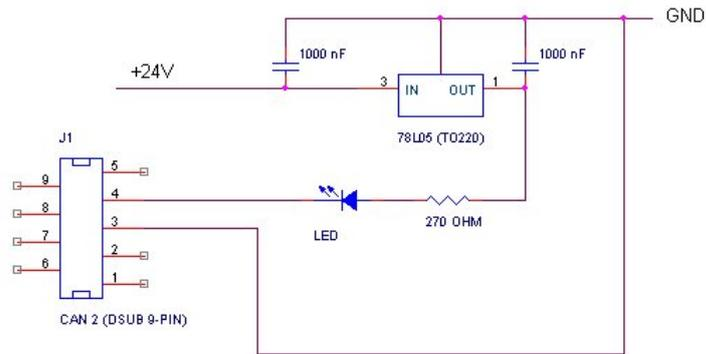
Figure 9: Sample circuit for connecting a LED to the External trigger output.
