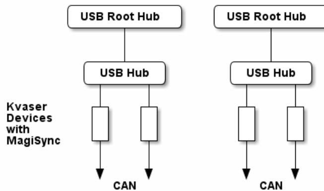
Figure 12: Not all devices are synchronized via MagiSync in this setup.
