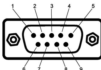
Figure 6: The D-SUB 9 connector pin numbers
